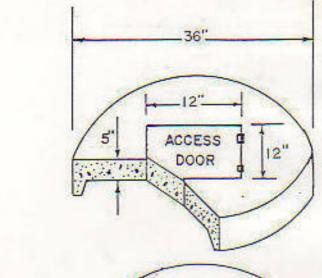
LID HAS NO.4 REBAR 12" O.C. w/6x6x10 WIRE MESH. FLAT TOP OPENINGS
